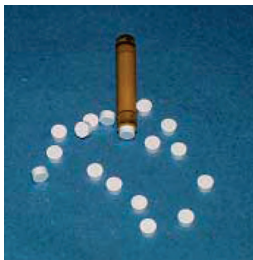
Figure 8 View of the rotor and tablets used to obtain spectra of formulated bambuterol hydrochloride (VIII).
